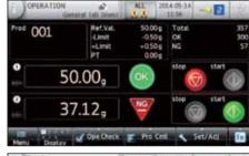
Statistical display of average weight and weight variations help the operator understand production trends for optimizing filling processes.
