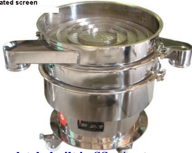
Completely built in SS w/casters for pharmaceutical application
